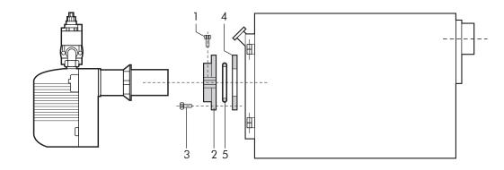
Fix flange 2 to the boiler using 4 screws 3 interposing the insulation gasket 4 and the possible insulating cord 5. Insert the burner in the flange so that the draught tube penetrates into the combustion chamber by the length suggested by the boiler manufacturer. Tighten screw 1 to lock the burner in position.
