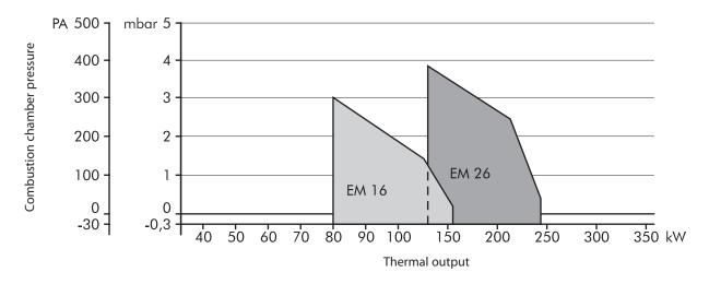
The pressure curves indicate the output in kW according to the backpressure in the combustion chamber, in mbars.
